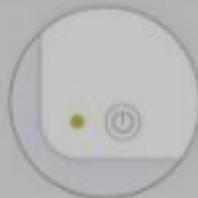
Power on the device and confirm that indicator light rapidly blinks
