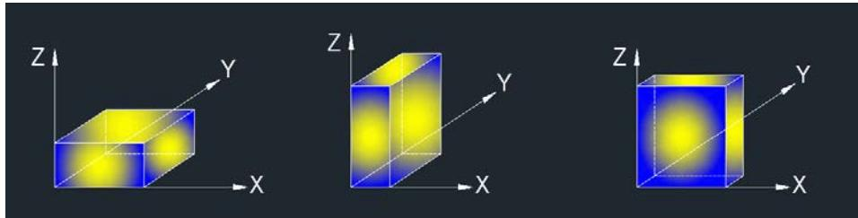
The fundamental of the EUT was investigated in three orthogonal axes X/Y/Z, it was determined that X axis was worst-case . Therefore, all final radiated testing was performed with the EUT in X axis.
