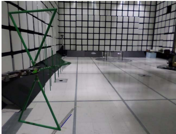
Figure 3: Radiated Emissions Limits, 30MHz-1000MHz - Setup Antenna View
