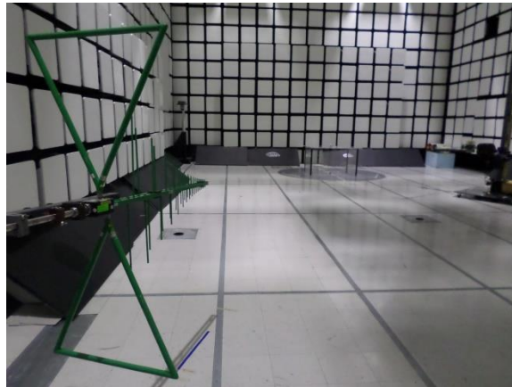
Figure 56: Radiated Emissions Limits, 30MHz-1000MHz - Setup Antenna View
