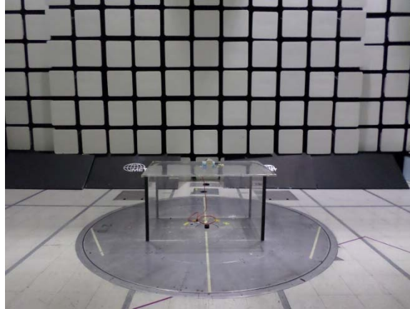
Figure 1: Radiated Spurious Emissions Test Setup, 30MHz-1000MHz - Setup Front View
