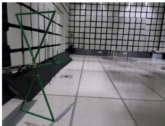
Figure 3: Radiated Spurious Emissions Test Setup, 30MHz-1000MHz - Setup Antenna View
