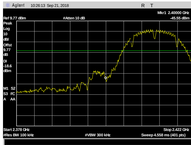
Plot 237. Conducted Band Edge, 802.11b, 2412 MHz, Low
