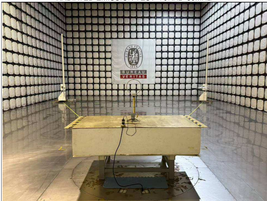
RADIATED EMISSION TEST < 9KHz~30MHz>
