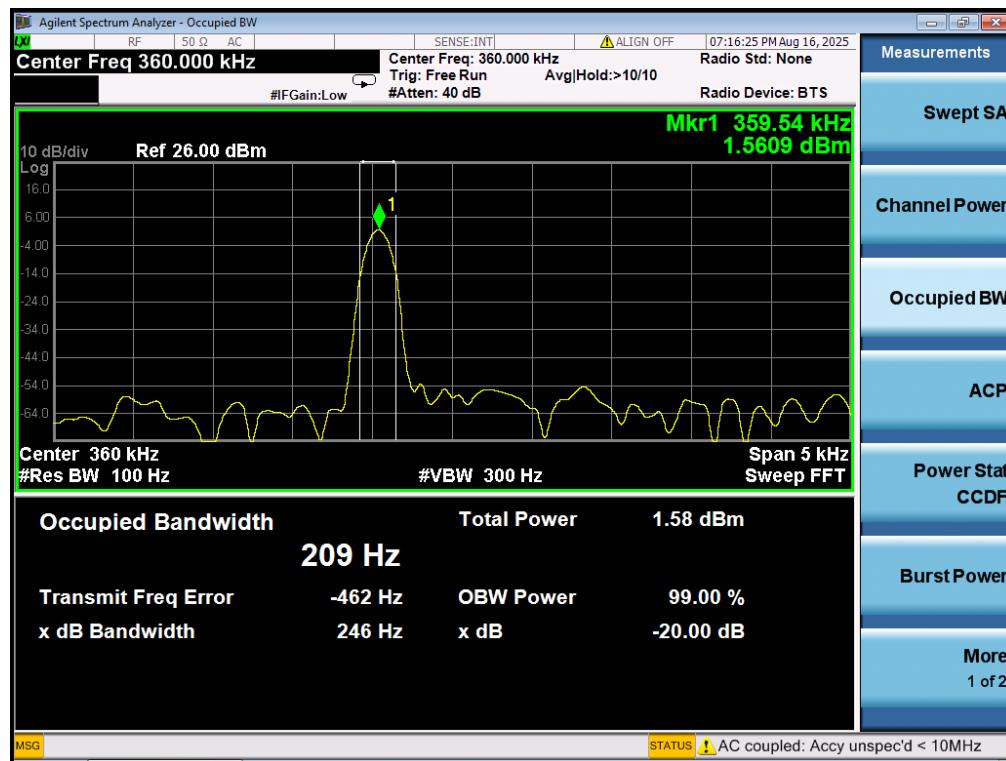
Note: Because the measured signal is CW-like, adjusting the RBW per C63.10 would not be practical since measured bandwidth will always follow the RBW and the result will be approximately twice the RBW.
