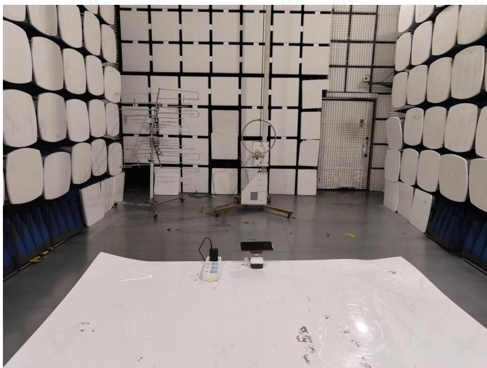
Radiated Emission below 30MHz-AC adapter charge mode
