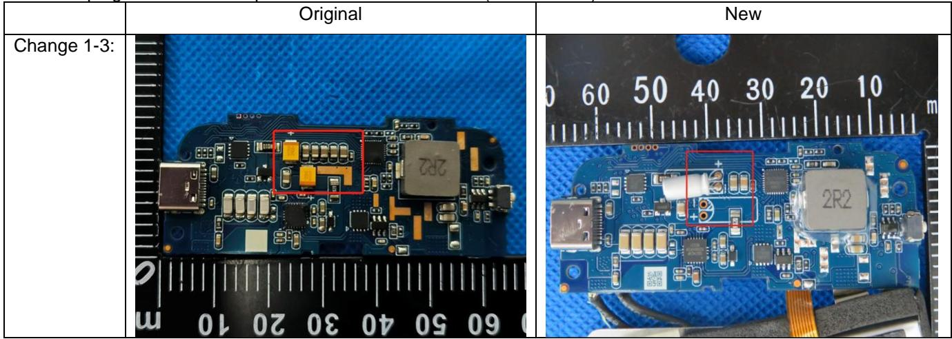
The change part of the circuit is discharge circuit, which does not affect the RF part.
