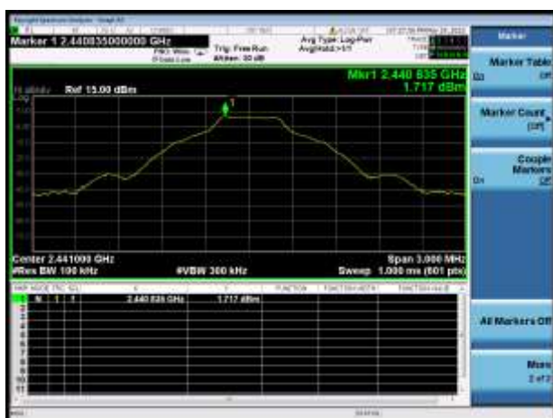
GFSK MIDDLE CHANNEL, CARRIER LEVEL
