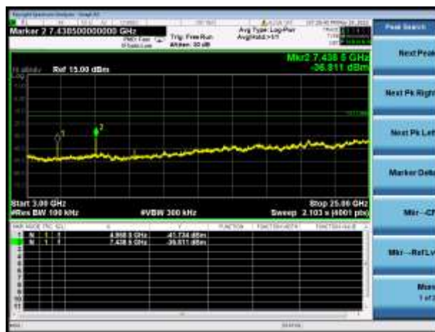
GFSK HIGH CHANNEL, SPURIOUS 3 GHz ~ 25 GHz
