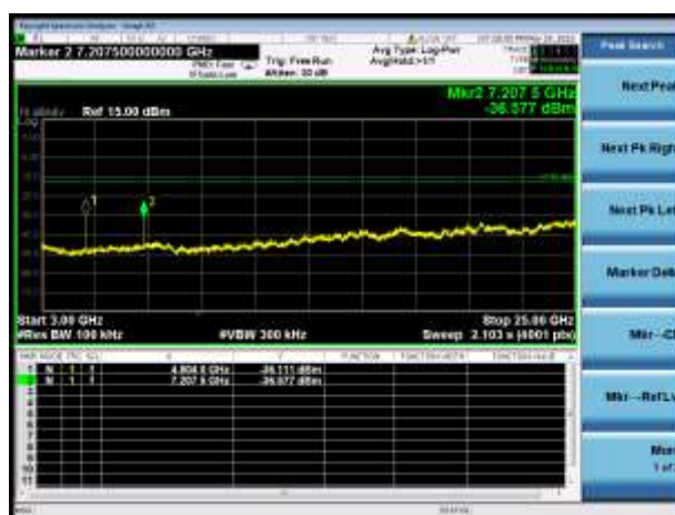
GFSK LOW CHANNEL, SPURIOUS 3 GHz ~ 25 GHz
