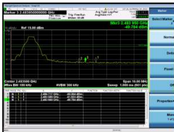
GFSK HIGH CHANNEL, BAND EDGE
