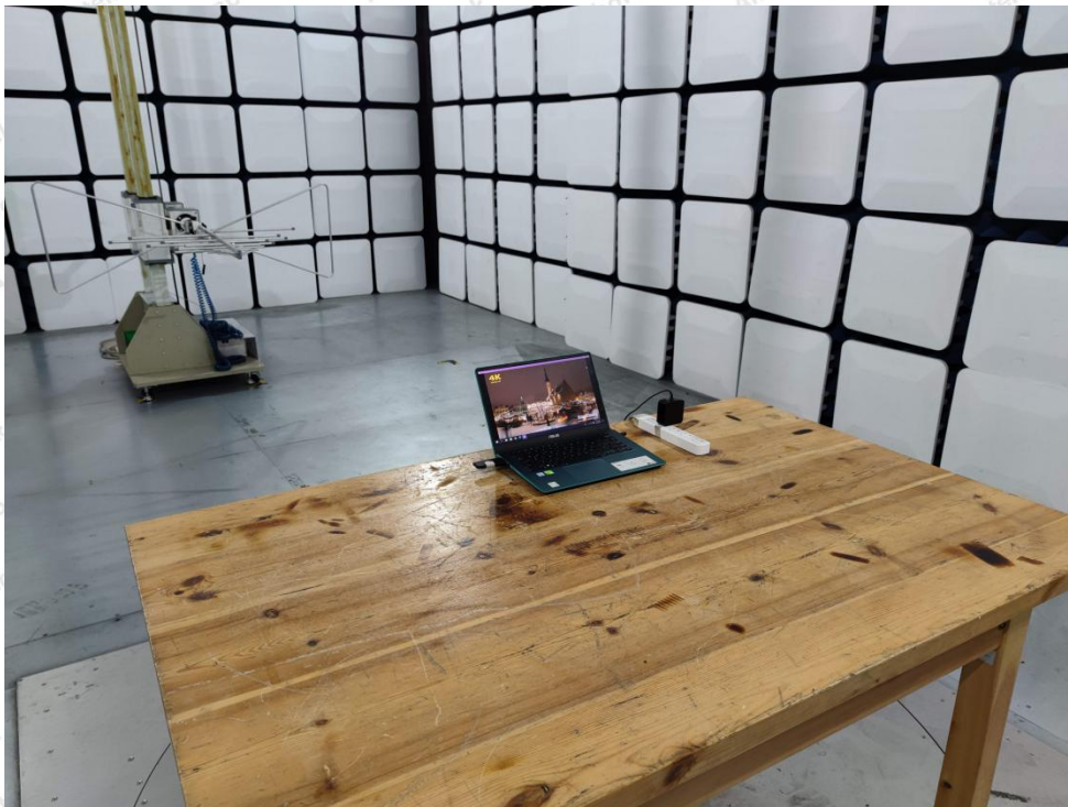
Photo of Radiation Emission Test
