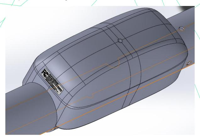
A sticker is placed on the housing with the measurements shown above. The adhesive is permanent acrylic adhesive and material of the sticker is durable Arlon 8000.
