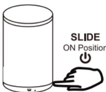
1. Slide the ON/OFF switch to the ON position to power on your speaker.
