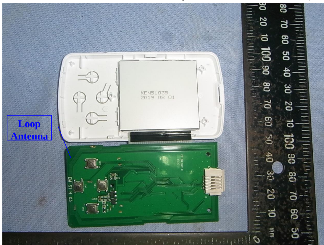
Figure 7 Internal View (LCD Panel and PCB Board, Back View)
