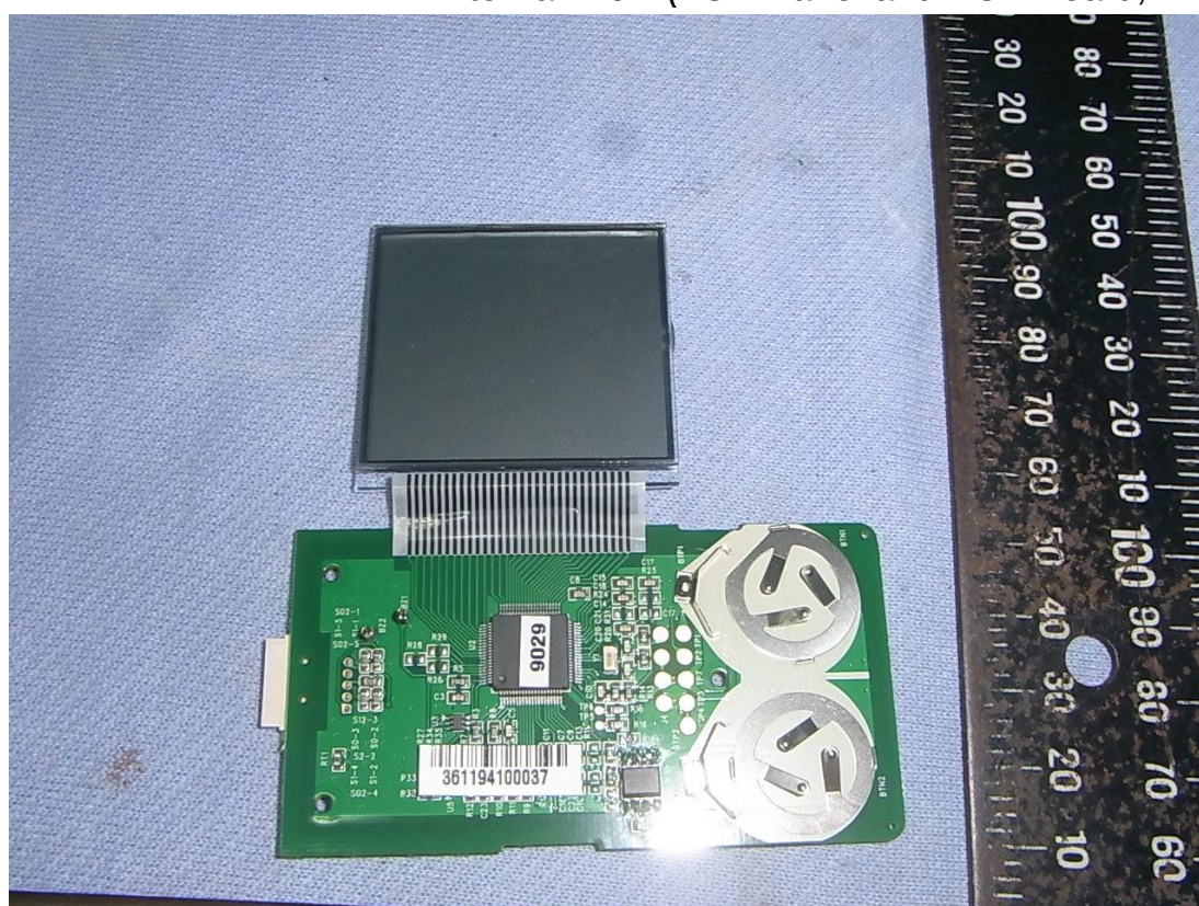
Figure 8 Internal View (LCD Panel and PCB Board, Front View)
