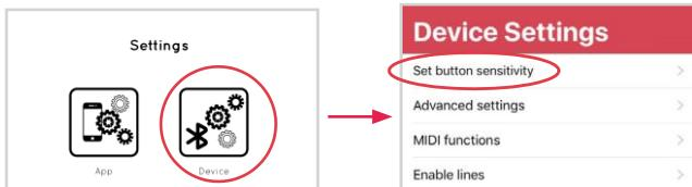
**Set button sensitivity** shows live capacitive touch signals for all the touch points.
