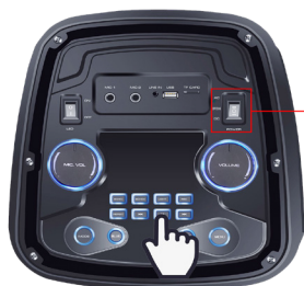
2. Press “Pause/Play” button for 3 seconds on one of the speakers to turn on/off the TWS function
