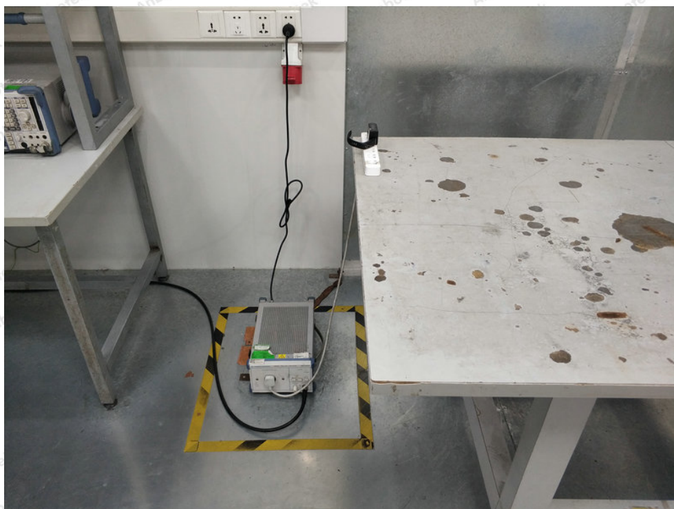
Photo of Conducted Emission Measurement
