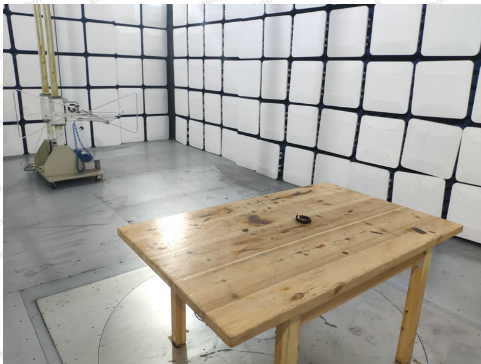
Photo of Radiation Emission Test
