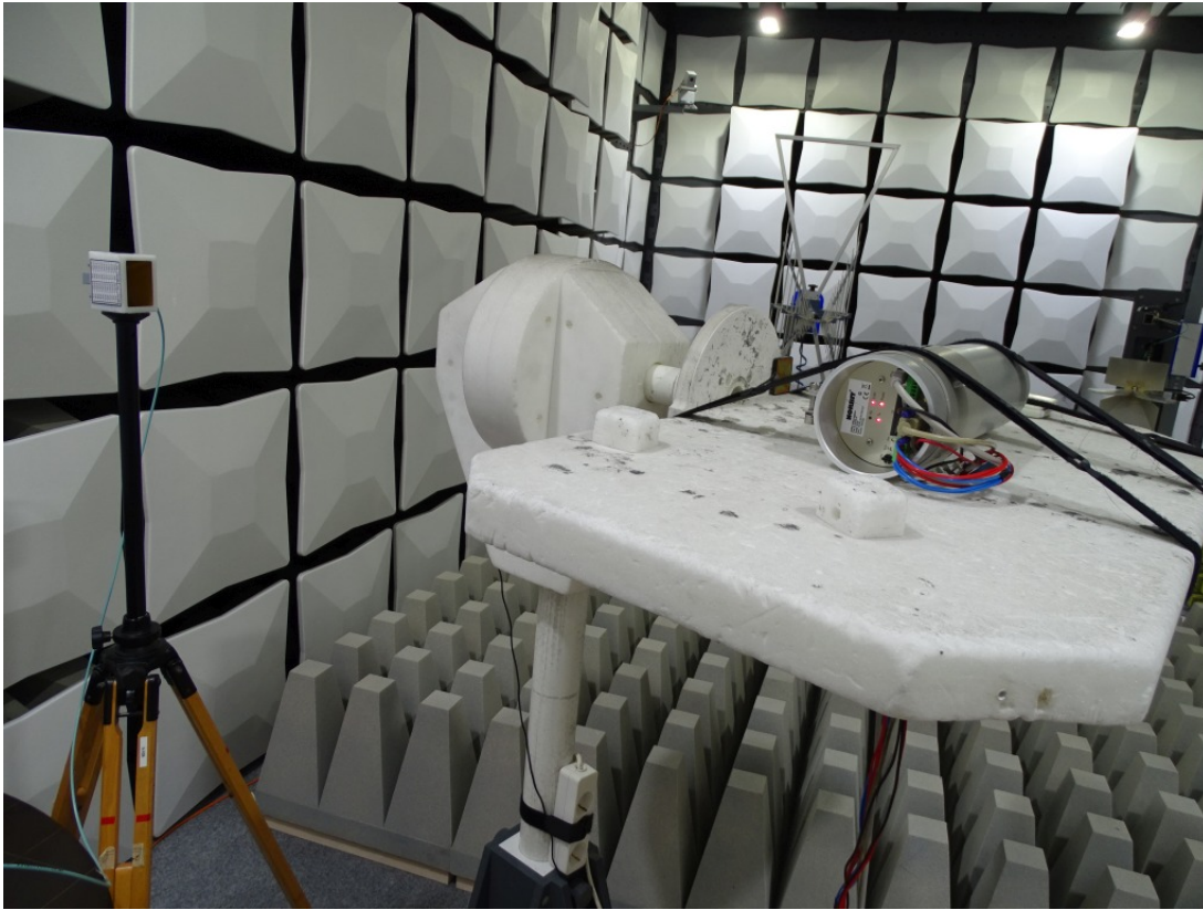
Photo 5: Test setup for radiated measurements (26 GHz – 40 GHz)
