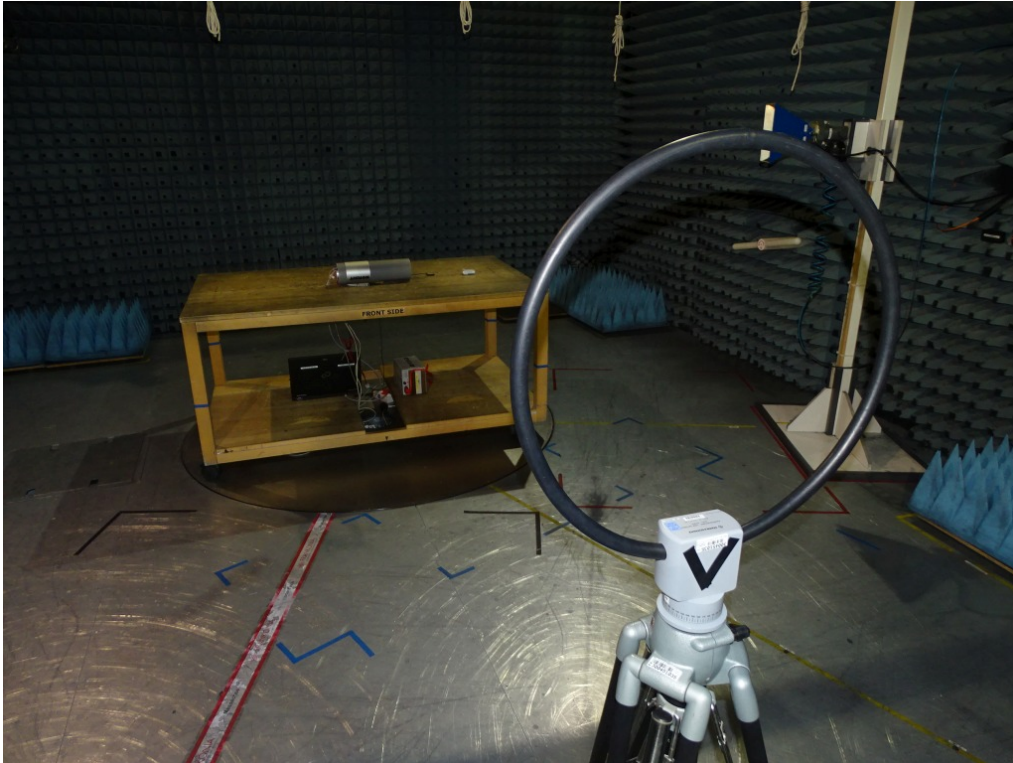
Photo 2: Test setup for radiated measurements (H-Field)
