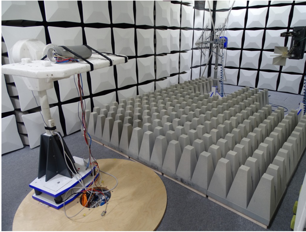
Photo 4: Test setup for radiated measurements (1 GHz – 26 GHz)
