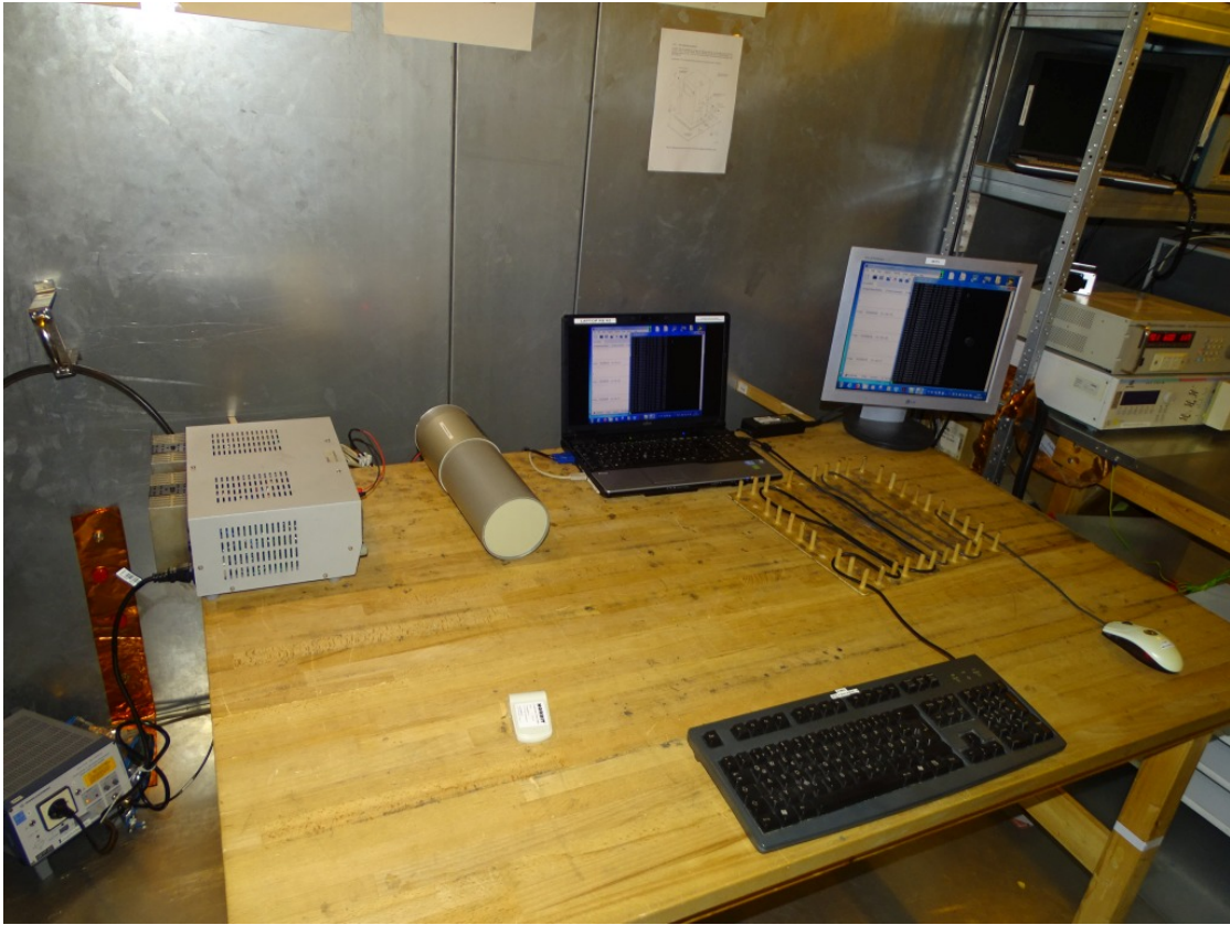
Photo 1: Test setup for conducted emissions at AC power line
