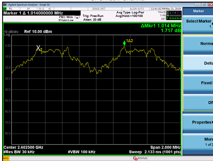
Test plots GFSK Low Channel
