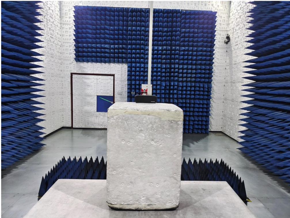
RADIATED EMISSION TEST SETUP ABOVE 1GHz
