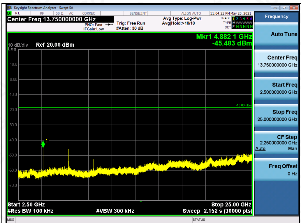
Test_Graph_EDR_ANT1_2441_2Mbps_Higher Band Emissions
