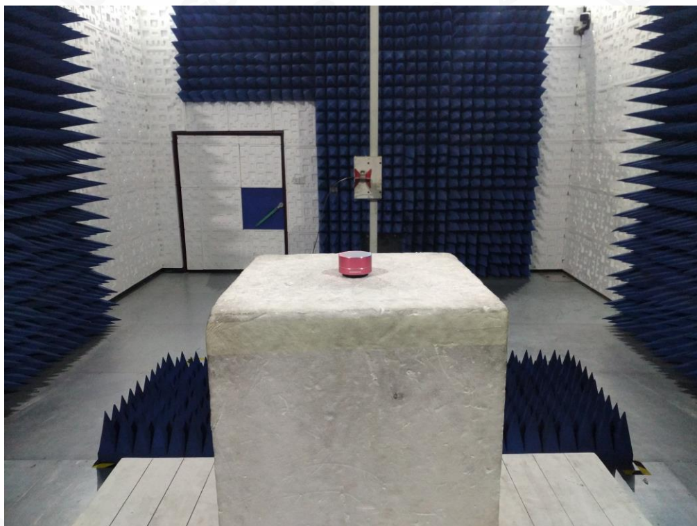
RADIATED EMISSION TEST SETUP ABOVE 1GHZ
