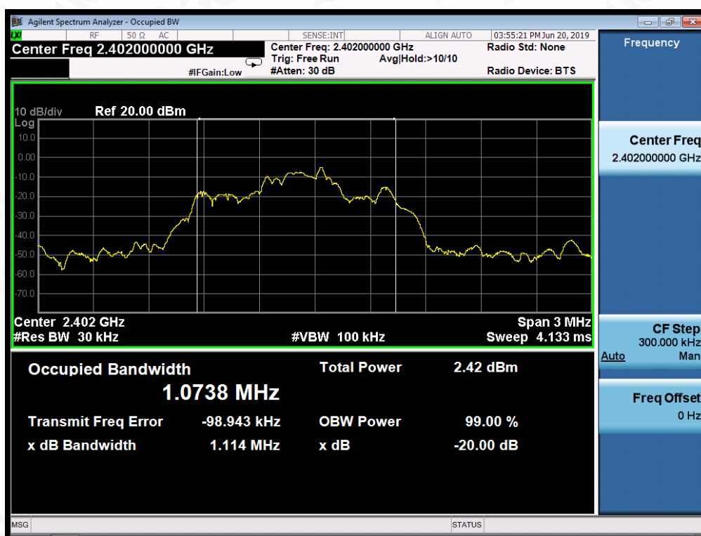
TEST PLOT OF BANDWIDTH FOR LOW CHANNEL
