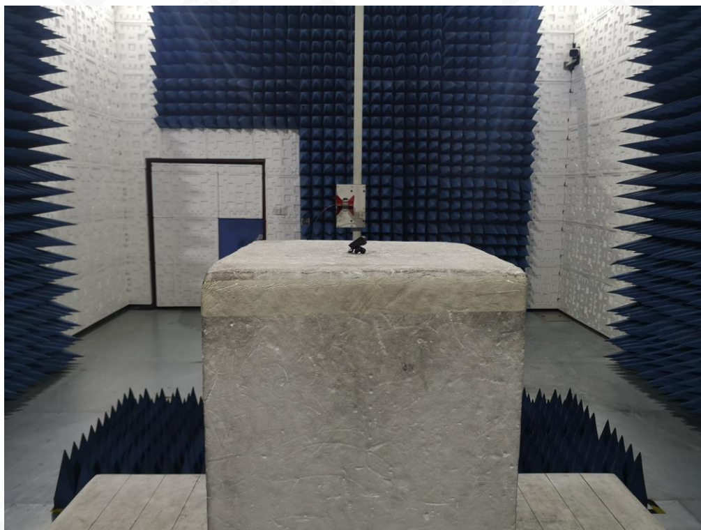
RADIATED EMISSION TEST SETUP ABOVE 1GHZ
