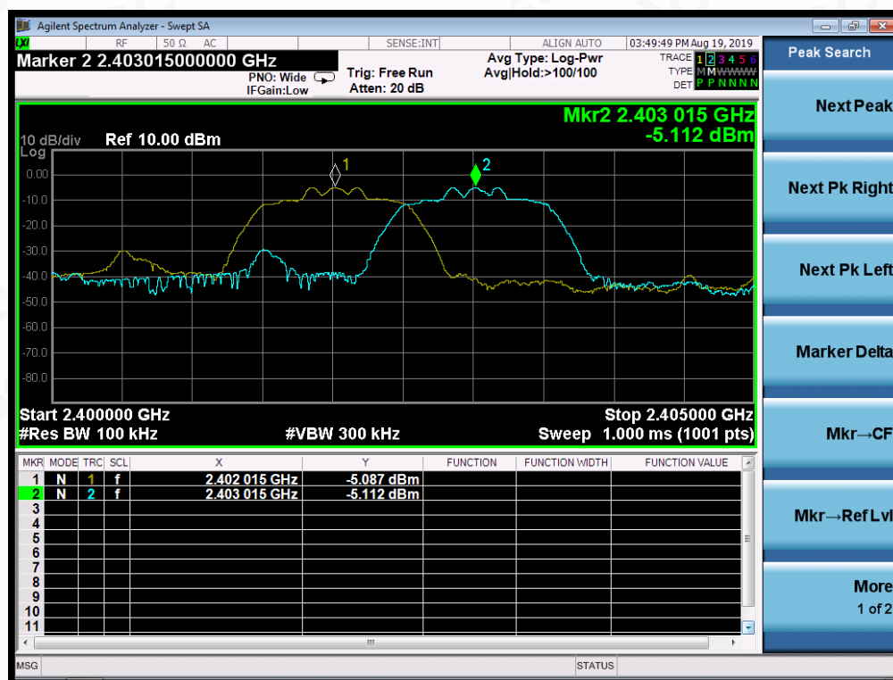
TEST PLOT FOR FREQUENCY SEPARATION
