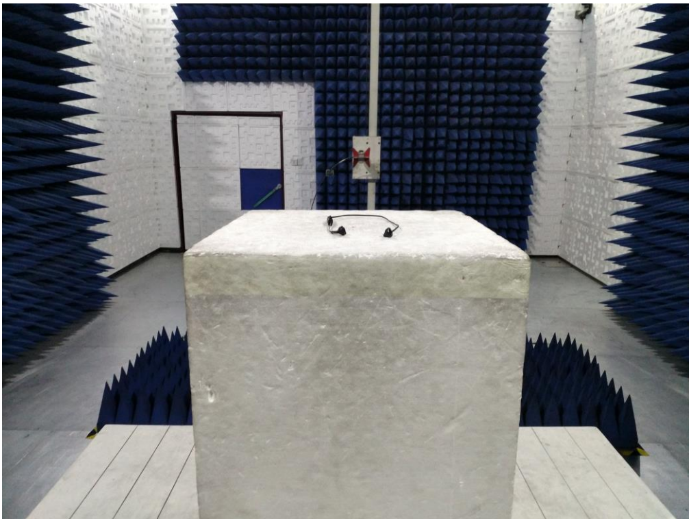
RADIATED EMISSION TEST SETUP ABOVE 1GHZ
