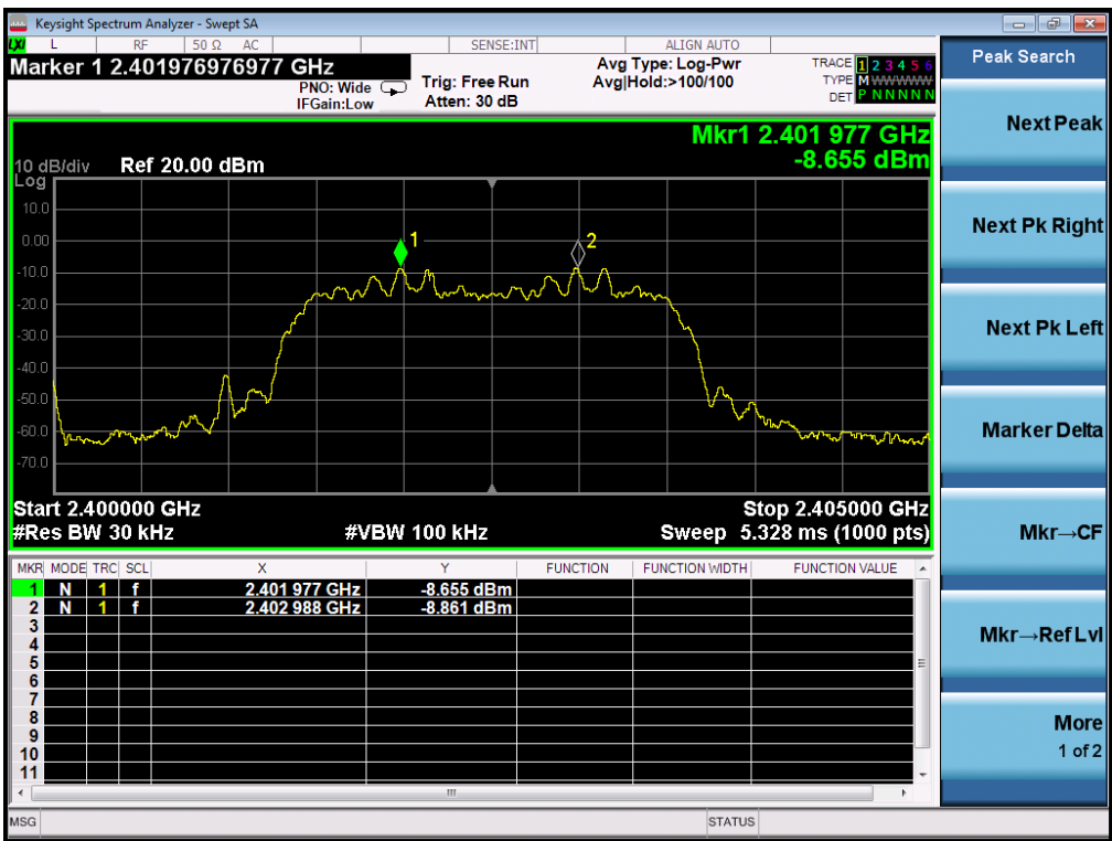
TEST PLOT FOR FREQUENCY SEPARATION
