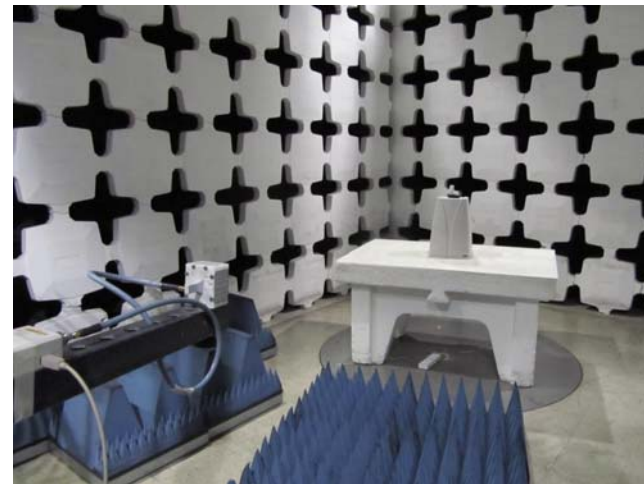
Radiated emissions test set above 18GHz.
