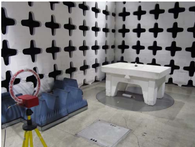
Radiated emissions test set up below 30MHz.
