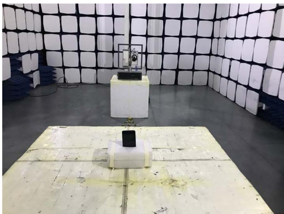
**Radiation Emission Test Setup (30MHz to 1GHz)**
