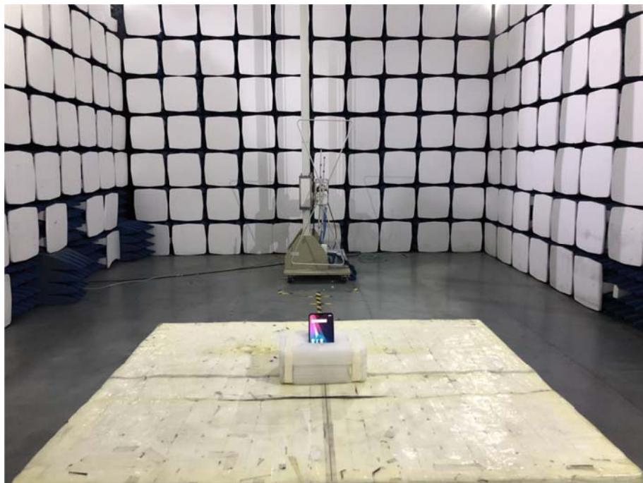
**Radiation Emission Test Setup (1GHz to 18GHz)**
