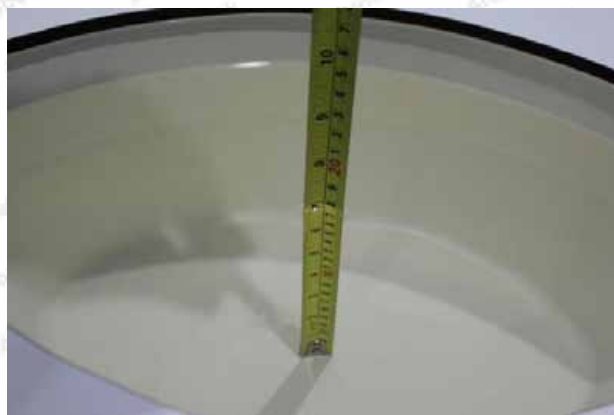
Liquid depth in the body phantom (5GHz)
