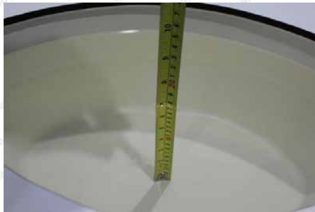
Liquid depth in the body phantom (5GHz)
