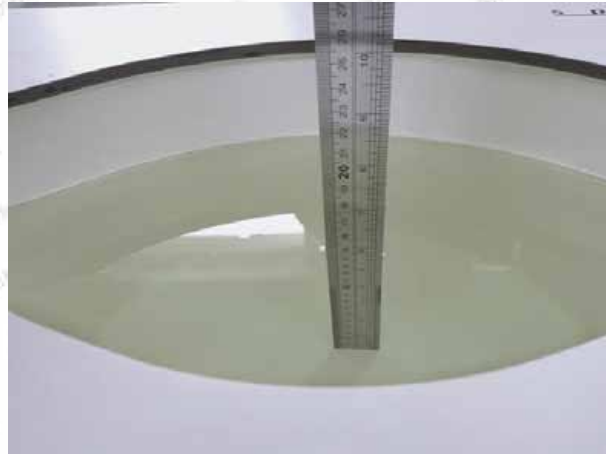
Liquid depth in the body phantom (2450MHz)
