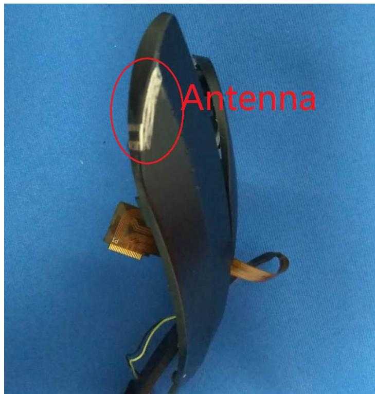
The antenna is integrated on the main PCB and no consideration of replacement. The best case gain of the antenna is 1.31dBi.
