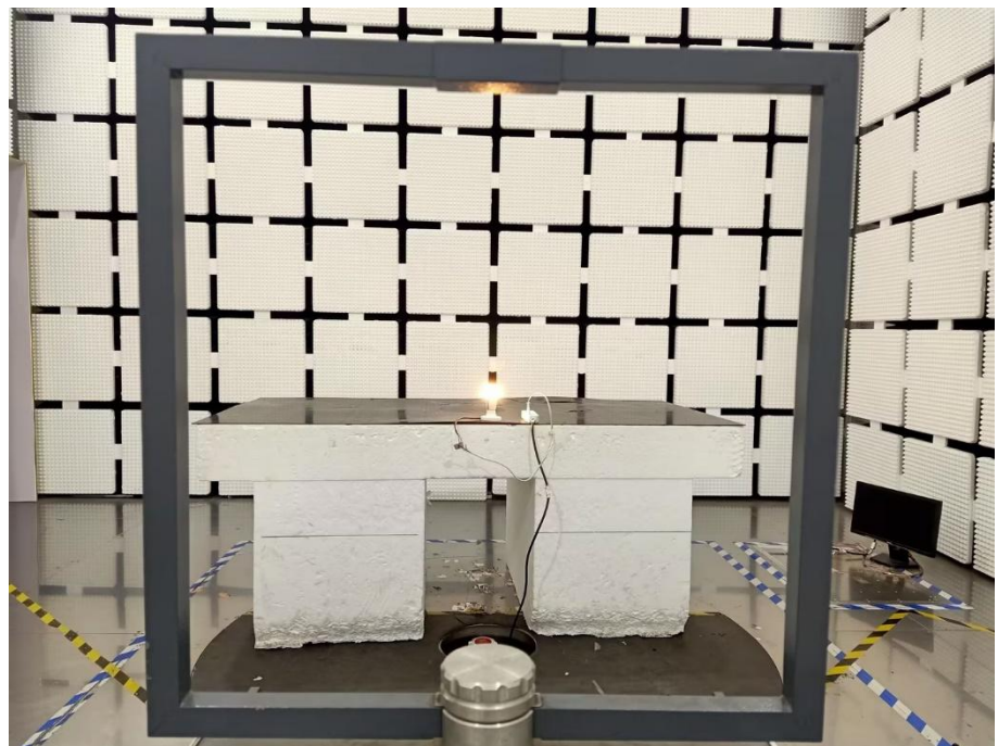
Radiation Emission Test Setup (Below 30MHz)
