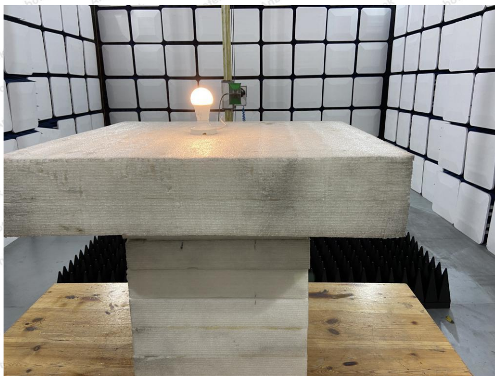
Photo of Radiation Emission Test
