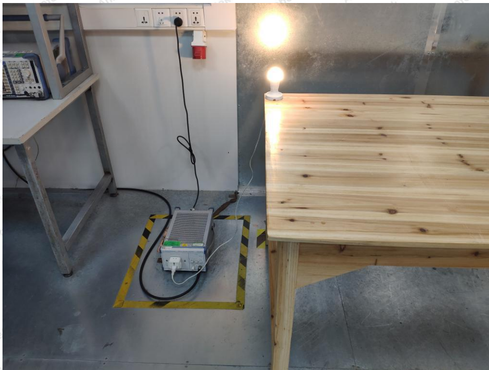
Photo of Power Line Conducted Emission Test
