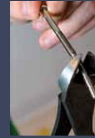
Note: Always cut the bolt at one of the cutting points so as not to damage a thread. Use the cutting edges of pins to grip strongly several times around the selected cutting point. If the cut produces a sharp point, please sand the tip of the bolt to smooth it out.
