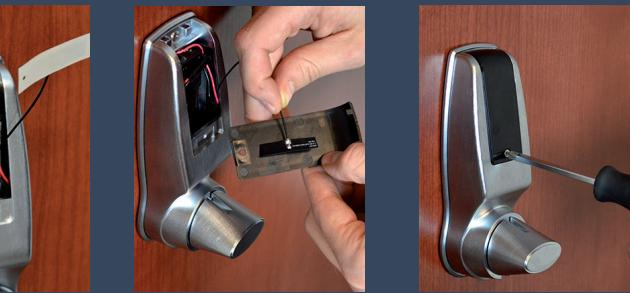
Once the battery pack is inserted, store any excess power cable within the compartment. The antenna can be left alone for now, as it will be connected to the black plastic cover. We suggest sticking it to the side furthest away from where the antenna originates...
