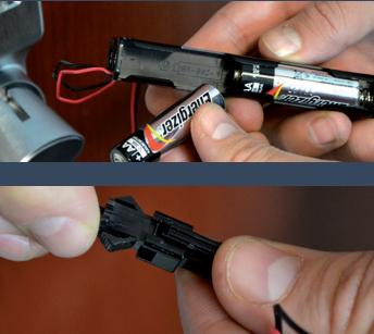
Once batteries are installed, connect the power cable from the lock to the battery pack.
