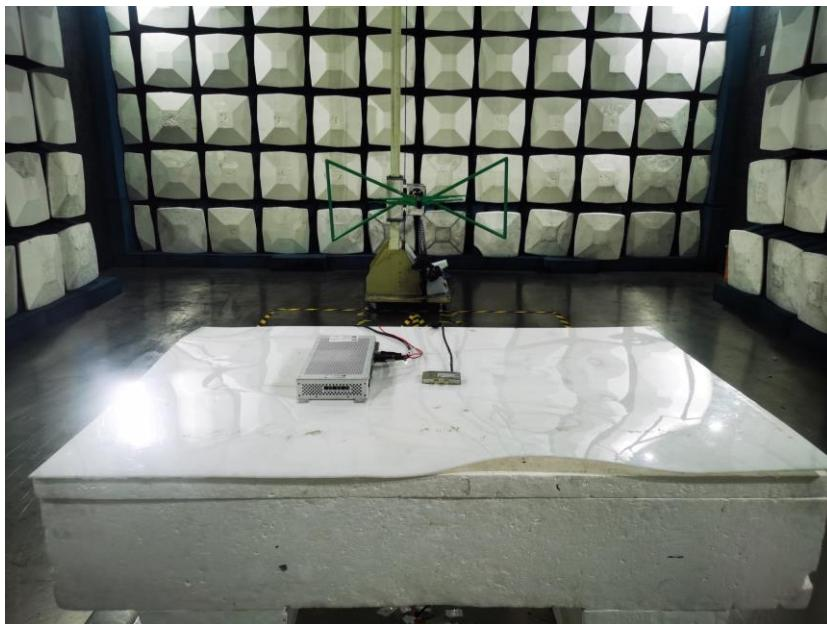
Radiated Spurious Emissions From 1GHz to 18GHz
