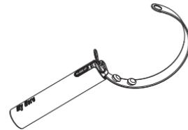
1. Insert a short side of a strap into a main cap at the top of a main body of the product as shown in the picture,
