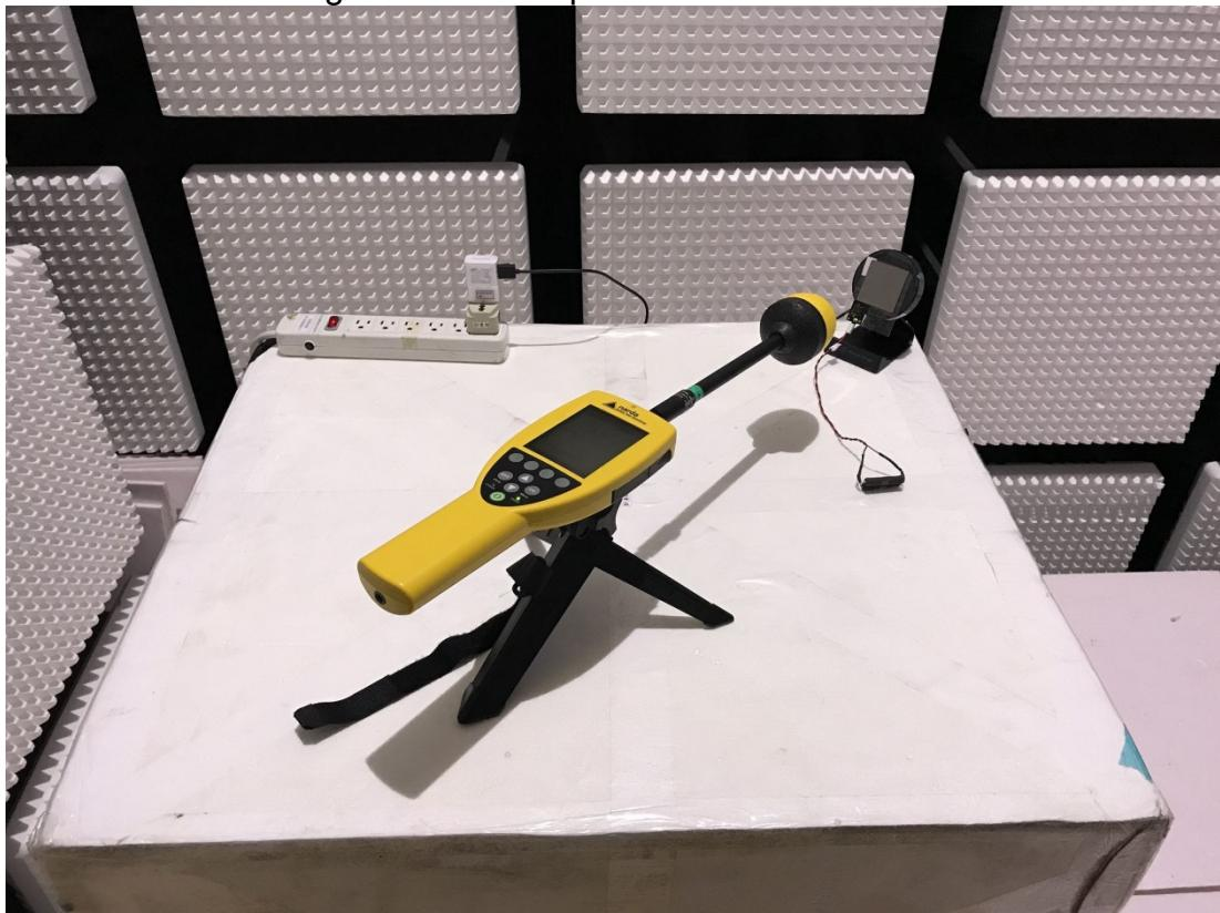
Test Mode: 10W Charge with AC Adapter
