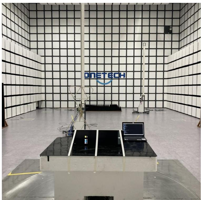
**- Radiated Emission Test (Above 1 GHz)**
