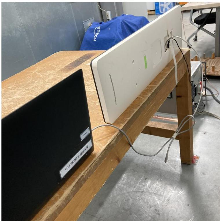
**- Radiated Emission Test (Below 1 GHz)**
