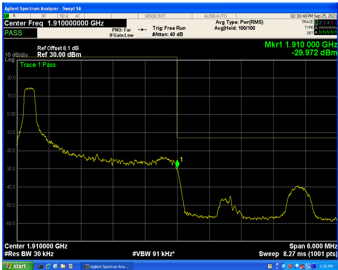
Band2 QPSK BW=3MHz Channel=19185 RB Size=15 Position=#0
