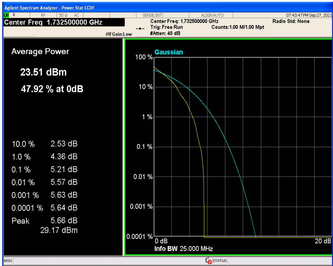
Band4 QAM16 BW=1.4MHz Channel=20175 RB Size=1 Position=#0
