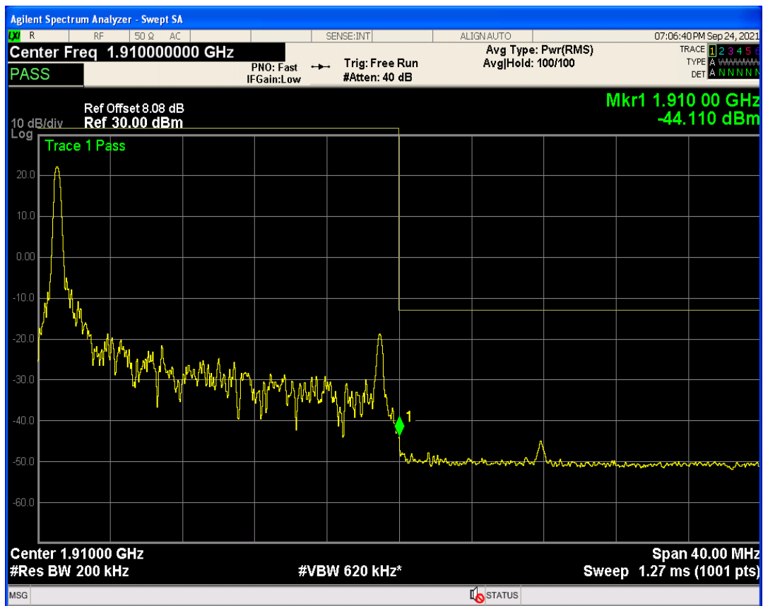
Band2 QAM16 BW=20MHz Channel=18700 RB Size=1 Position=#Max
