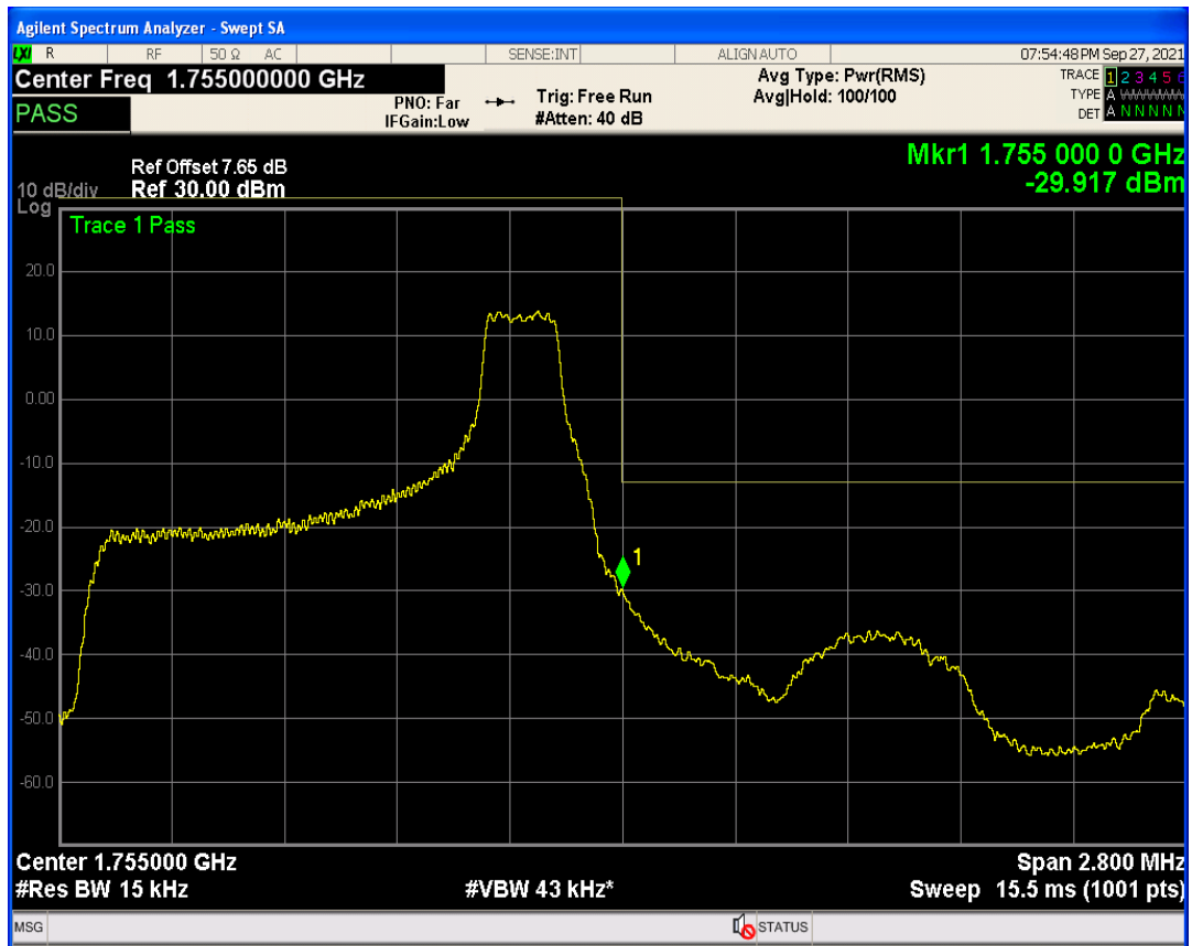
Band4 QAM16 BW=1.4MHz Channel=20393 RB Size=1 Position=#0
