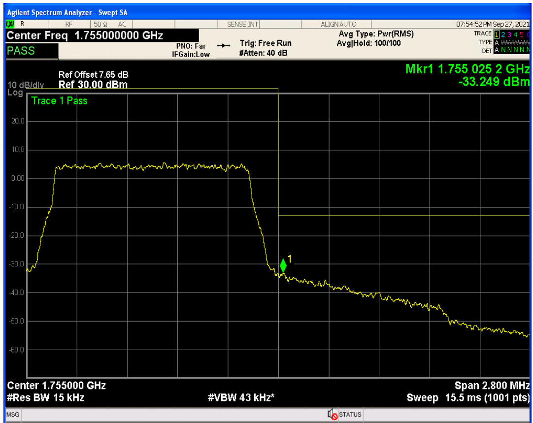
Band4 QAM16 BW=1.4MHz Channel=20393 RB Size=1 Position=#Max
