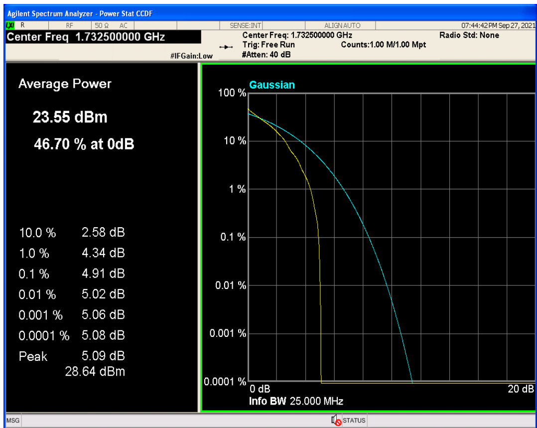
Band4 QAM16 BW=15MHz Channel=20175 RB Size=1 Position=#0
