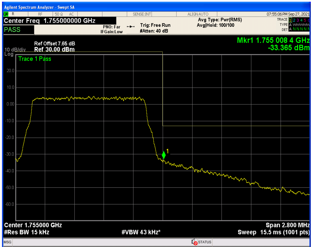
Band4 QPSK BW=3MHz Channel=19965 RB Size=1 Position=#0
