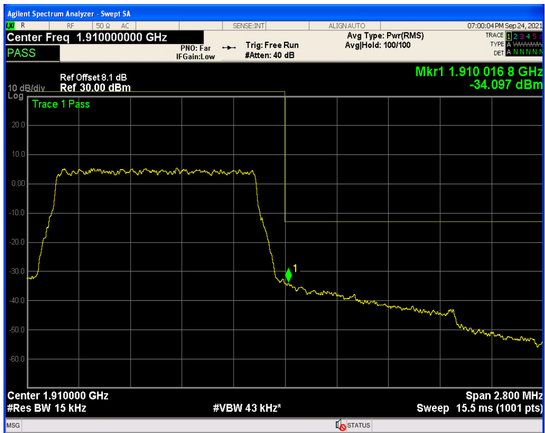
Band2 QAM16 BW=1.4MHz Channel=19193 RB Size=1 Position=#0
