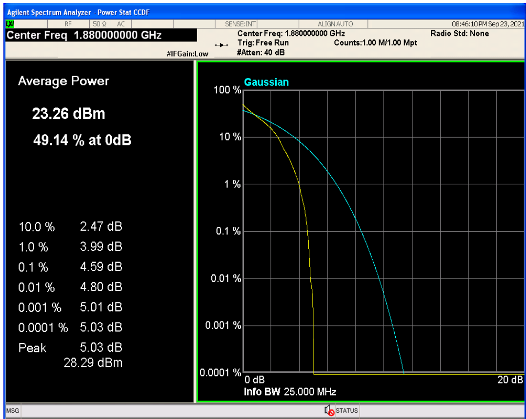
Band2 QAM16 BW=15MHz Channel=18900 RB Size=1 Position=#0
