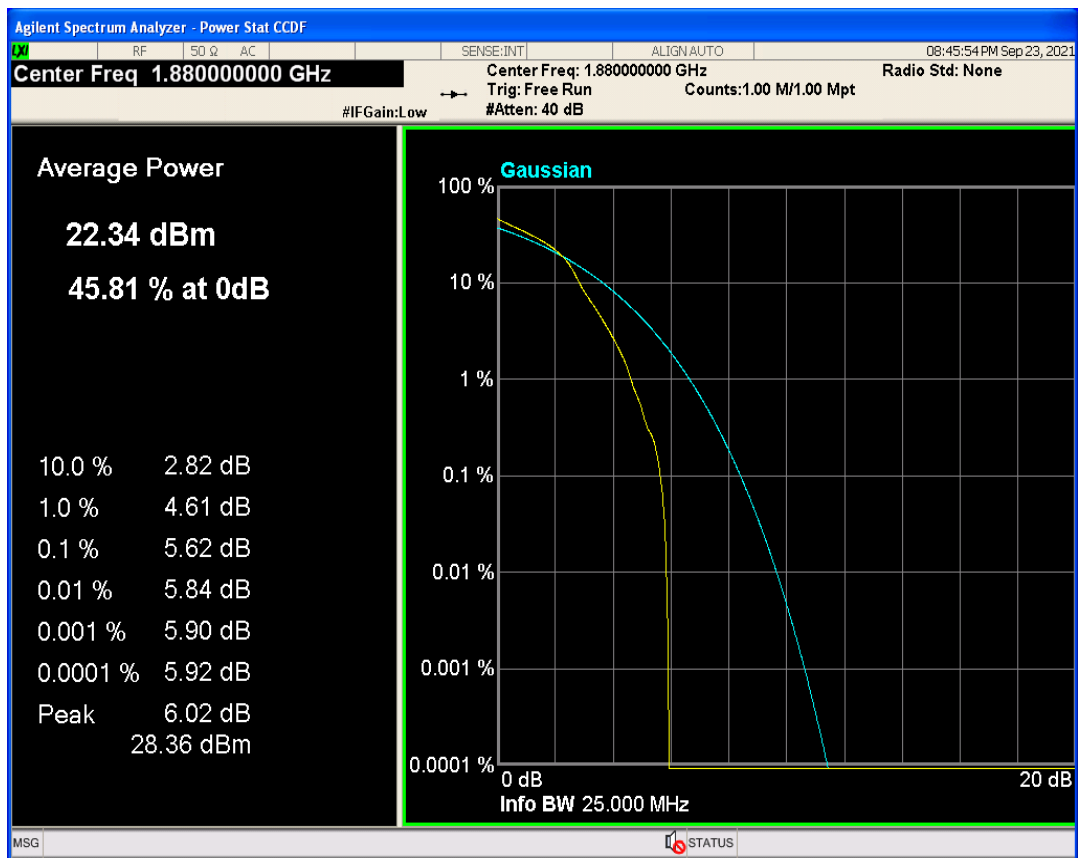
Band2 QPSK BW=15MHz Channel=18900 RB Size=1 Position=#0
