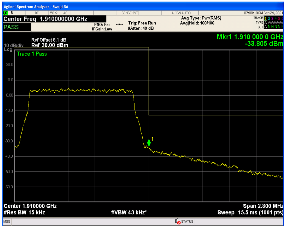
Band2 QPSK BW=3MHz Channel=18615 RB Size=1 Position=#0
