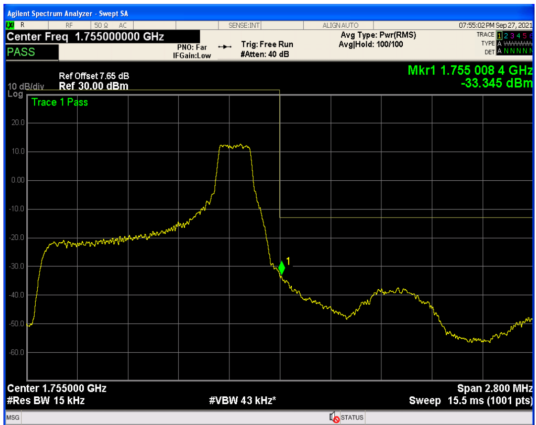
Band4 QAM16 BW=1.4MHz Channel=20393 RB Size=6 Position=#0
