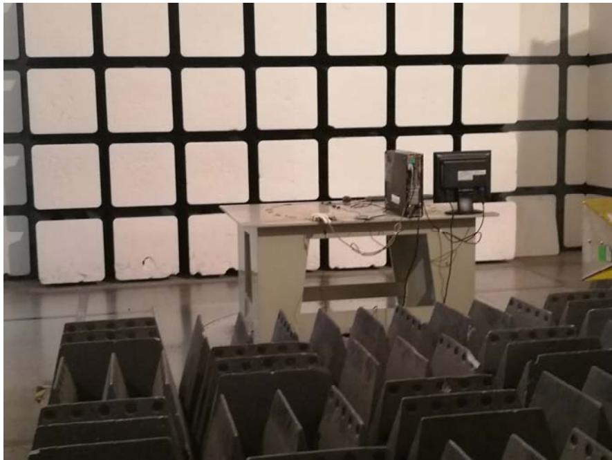
Radiated Emissions – Rear View (Above 1 GHz)
