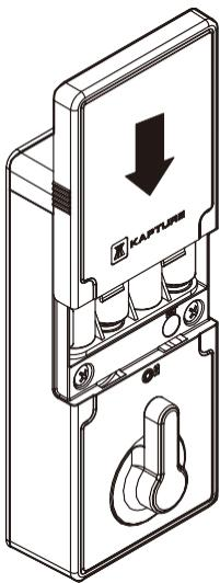
If the batteries have been installed correctly, then replace the battery cover. Kapture will then lock and unlock itself until it is calibrated.
