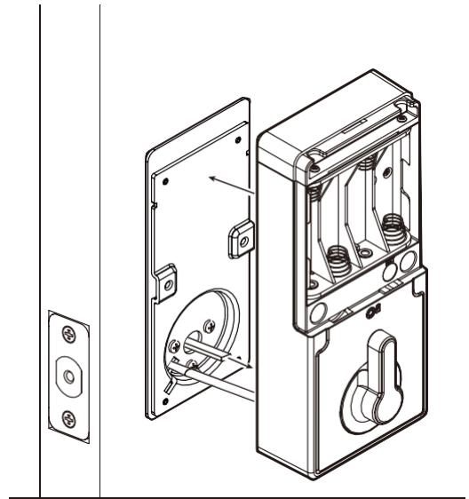
Turn the tailpiece until it's horizontal, to extend the deadbolt. Insert the tail piece into the slot on the back of the interior units. Lift the interior unit onto the backplate.
