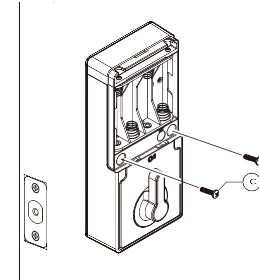
Use screws (C) at the interior unit to secure it to the backplate on the inside of the door.
