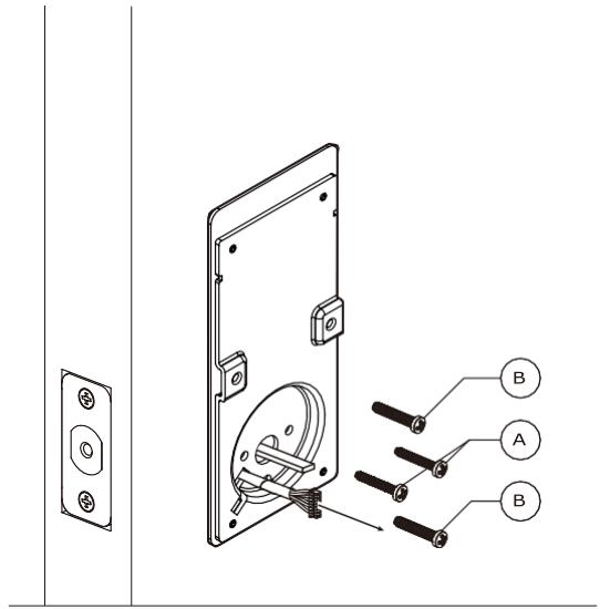
Use two (B) machine screws and two (A) narrow machine screws to secure the backplate to the keypad unit.
