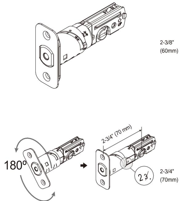
The latchbolt is preset at the factory with a 2-3/8" (60mm) backset. If a longer backset is needed, rotate the head as shown to extend it to a 2-3/4" (70mm) backset.
