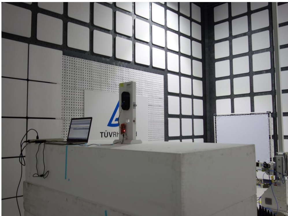
Photograph 4: Set-up for Spurious Emissions (Back View 2)
