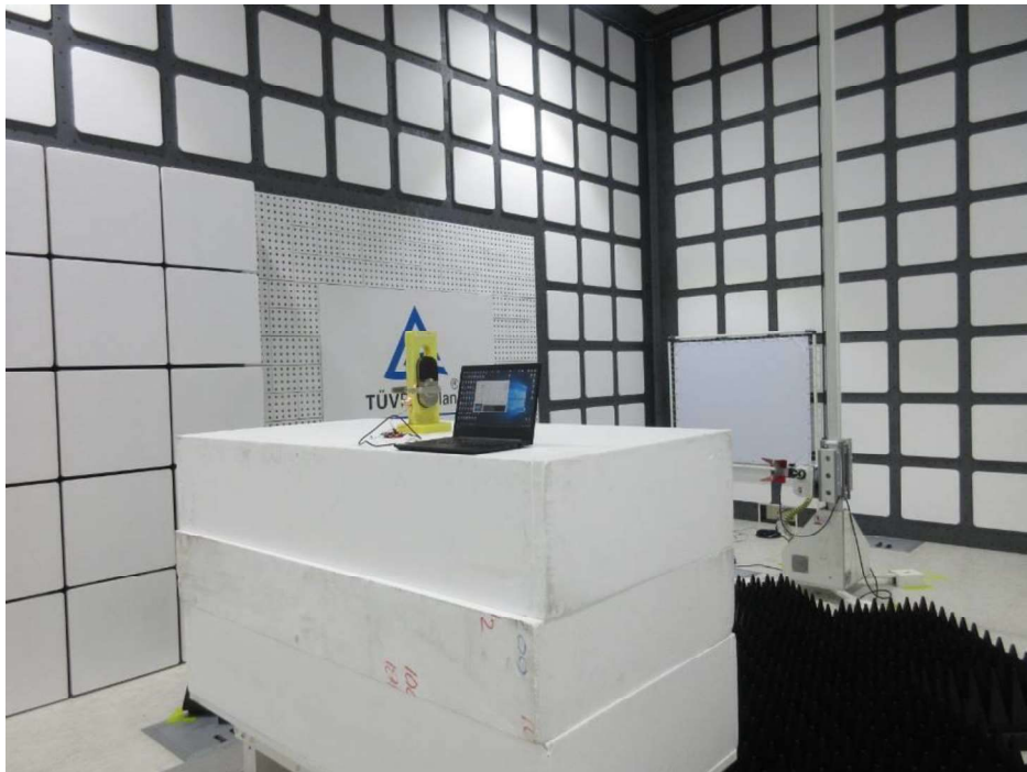
Photograph 4: Set-up for Spurious Emissions (Back View 2)
