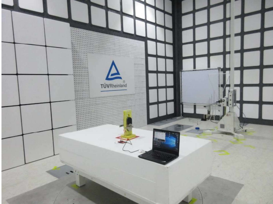
Photograph 3: Set-up for Spurious Emissions (Back View 1)
