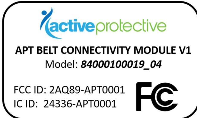
As the device is small in size, this label is provided in the module's user manual in lieu of physical application to the actual device.
