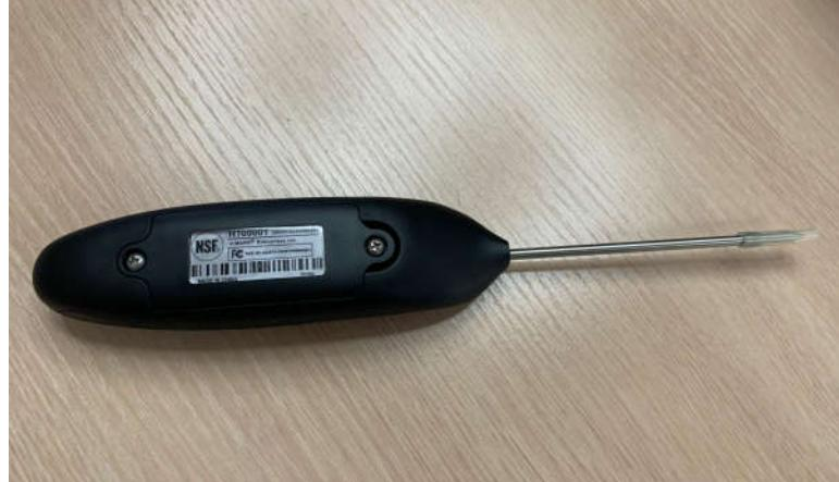
The label on the battery cover is retained (because inside the battery cover, the label can be prevented from wearing and falling off)
