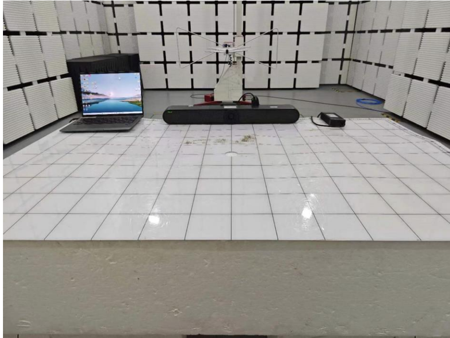
Set-up for Radiated Spurious Emission, Above 1GHz
