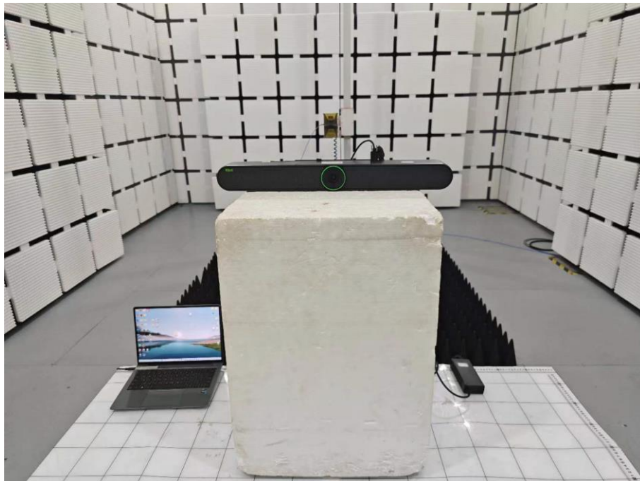
Set-up for Radiated Spurious Emission, Above 1GHz
