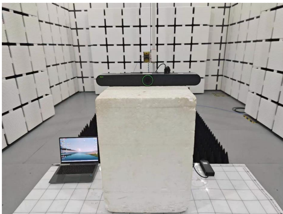
Set-up for Radiated Spurious Emission, Above 1GHz
