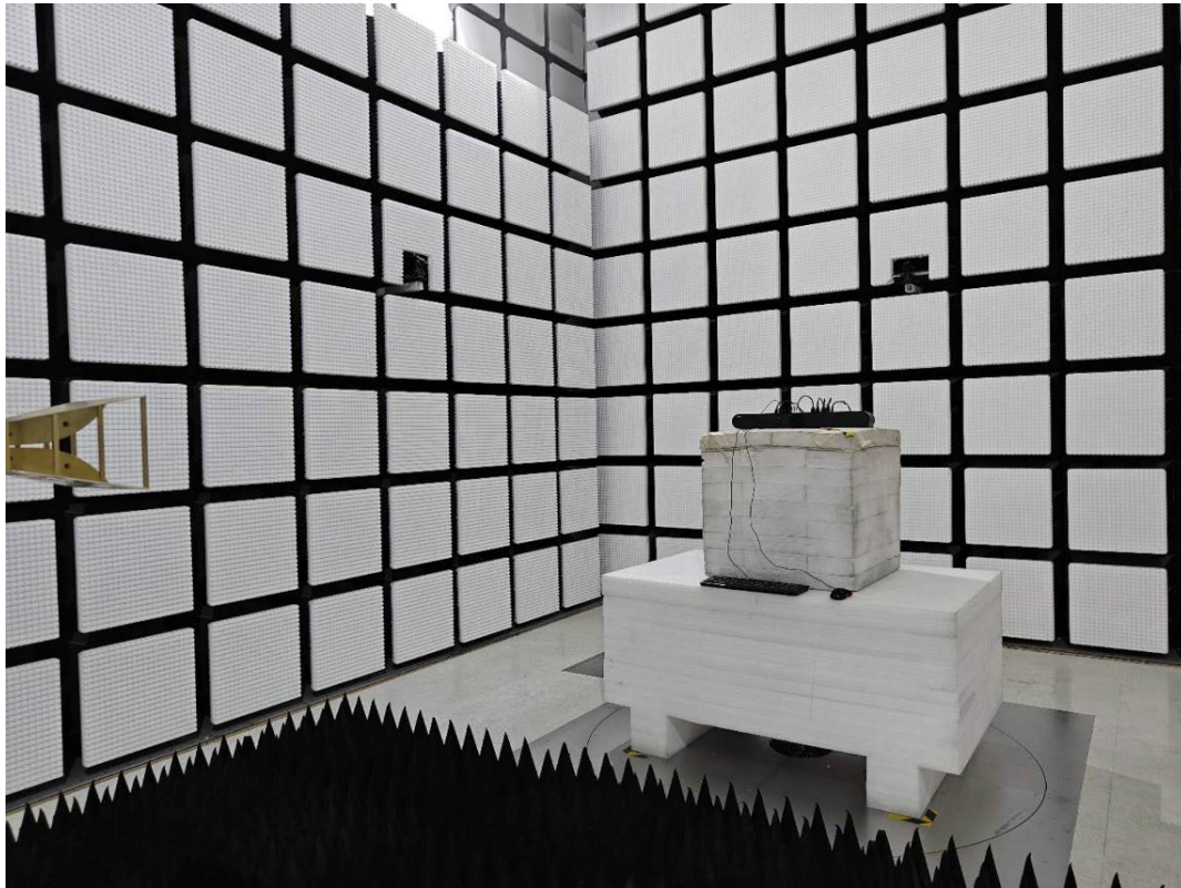
Radiated Emission 18-26.5GHz View
